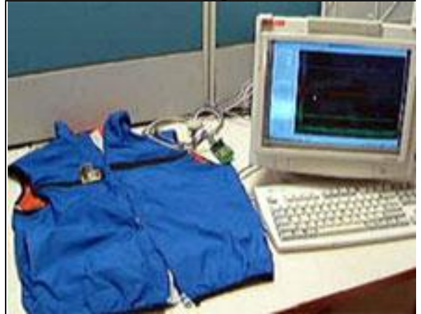
The jacket is fitted with a sensor and a Bluetooth transmitter that communicates with a receiver.
